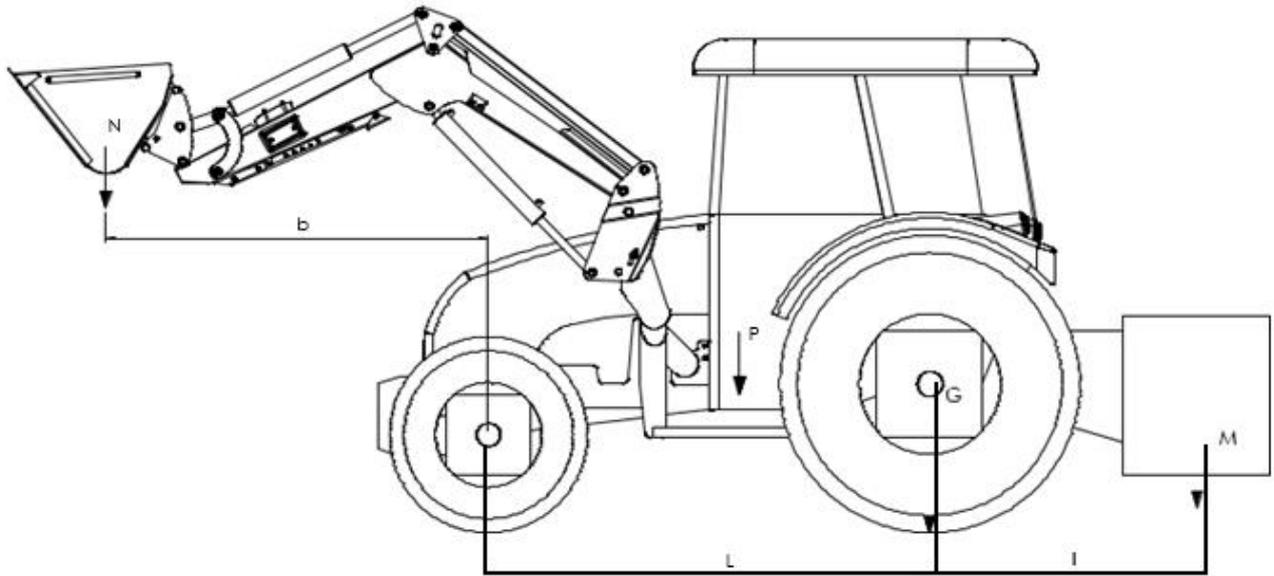
**Figure 11.** Loader-Tractor System Stability
