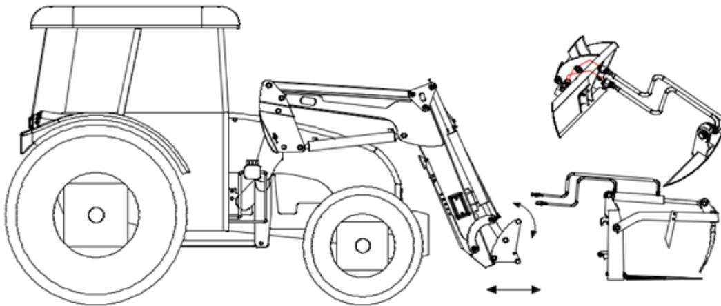
**Figure 20.** Installation of a tool that requires connection to the Loader's hydraulic system
