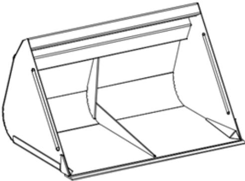
**Figure 23.** Loose material bucket
