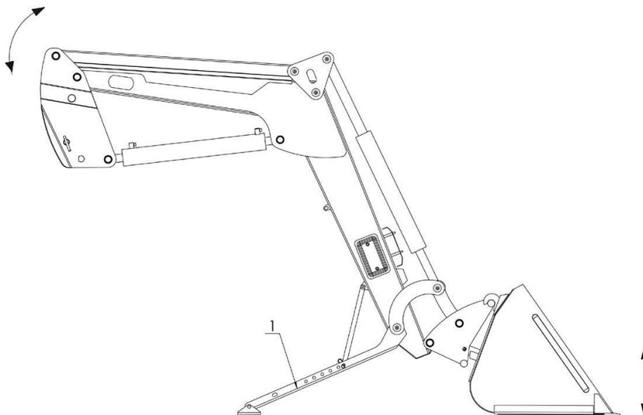
**Figure 10.** Attaching the Loader to a tractor.
