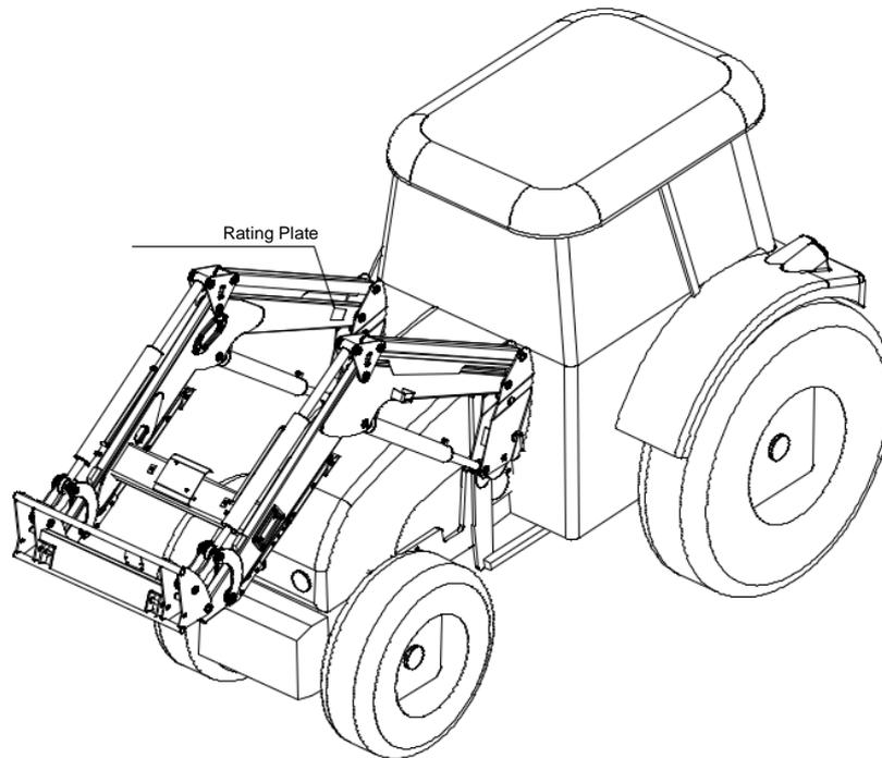
**Figure 2.** Location of the rating plate on the machine
