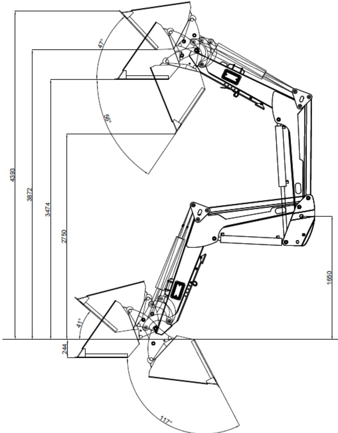
**Figure 7.** The dimensions of the T248 Loader installed on the tractor with a mounting point of 1650 mm above the ground
