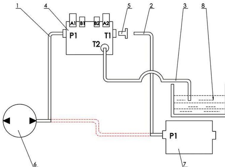
**Figure 16.** General diagram of the Loader's hydraulic connections.
