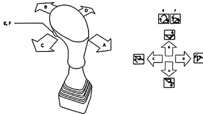
**Figure 13.** Control functions of the Loader control lever
