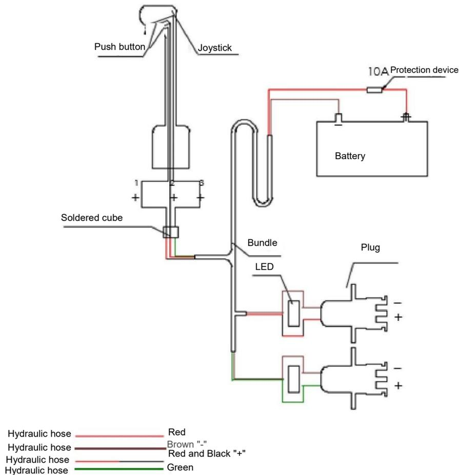
**Figure 15.** Loader's electrical installation wiring diagram.
