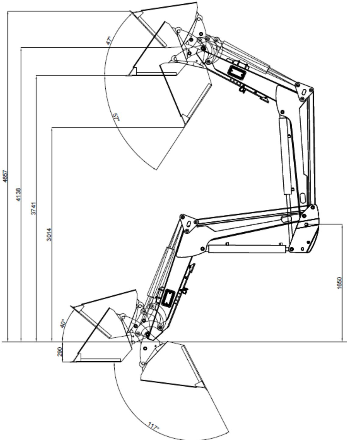
**Figure 8.** The dimensions of the T248D Loader installed on the tractor with a mounting point of 1650 mm above the ground
