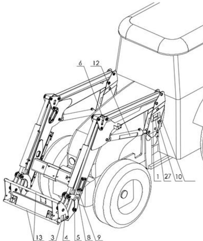
**Figure 6.** Pictograms arrangement on the machine – left side
