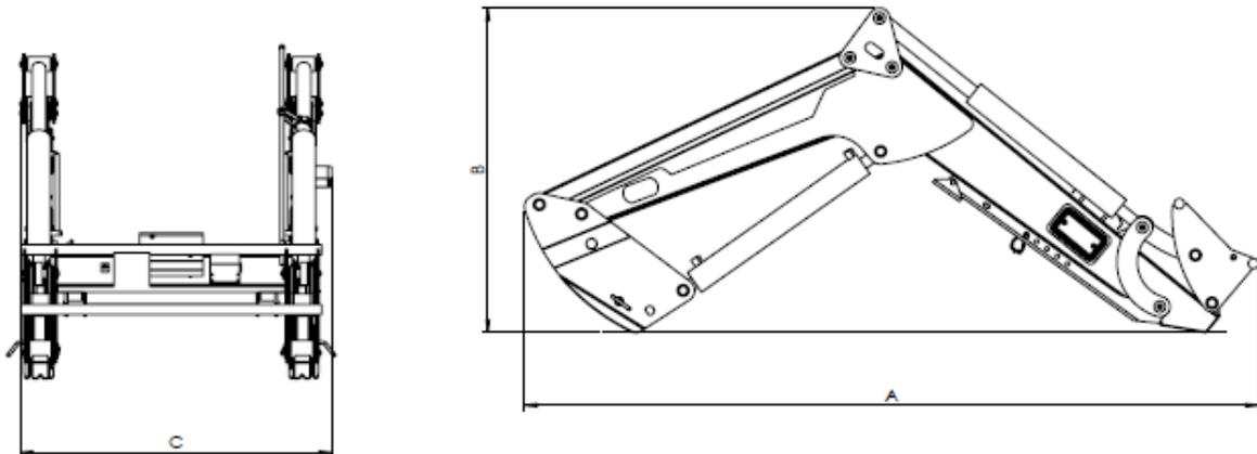
**Figure 43.** Dimensions of the Loader prepared for transport
